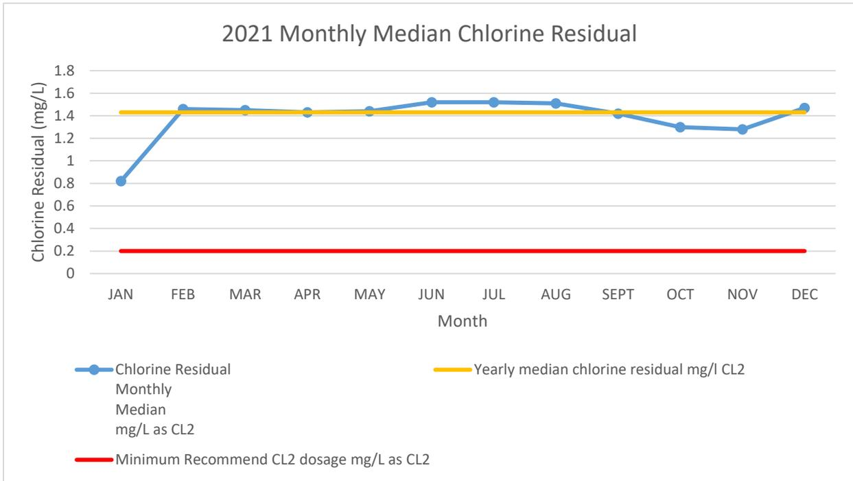
Figure 1 - 2021 Monthly Median Chlorine Residual
